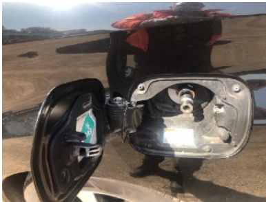
Cap over receptacle removed
